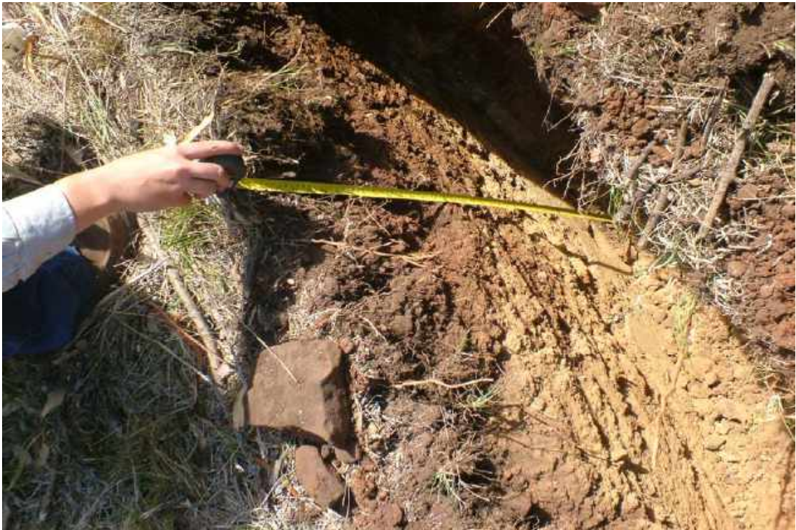
Plate 1: Typical Soil Profile from Test Pit
